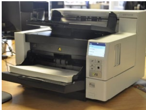
Fig. 4 Document scanner for destructive scanning
